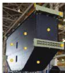
and demonstrating damage arresting composites technology in a Pultruded Rod Stitched Efficient Unitized Structure (PRSEUS).
