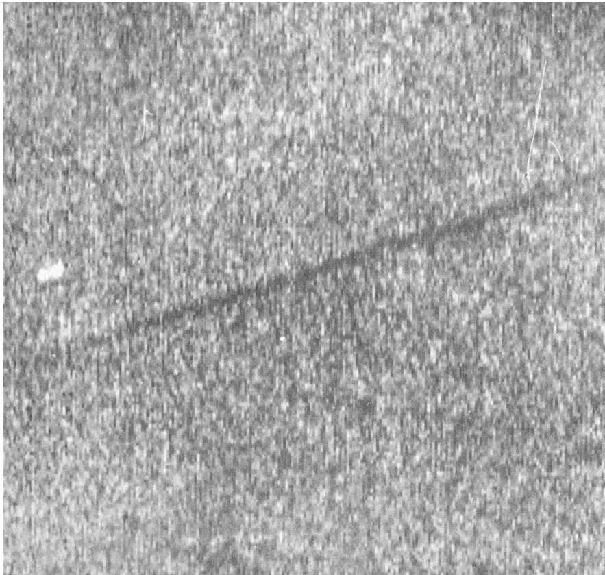
Figure 9.17 Azimuth shift in a SAR image. The image of the moving ship (the bright rectangular region, left centre) is displaced from the image of its wake (the dark diagonal stripe). (Image reproduced from Wahl et al. (1986) by courtesy of the European Space Agency.)
