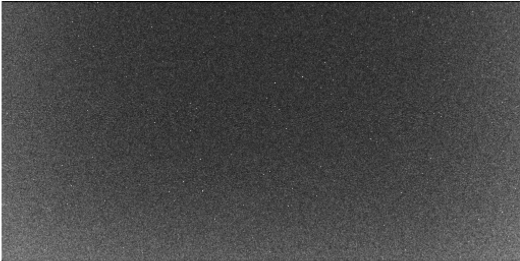
Figure 9.3.3 D(x,y) from Eq. (9.3.2) which shows how a typical dark image appears after it has been shutter corrected.
